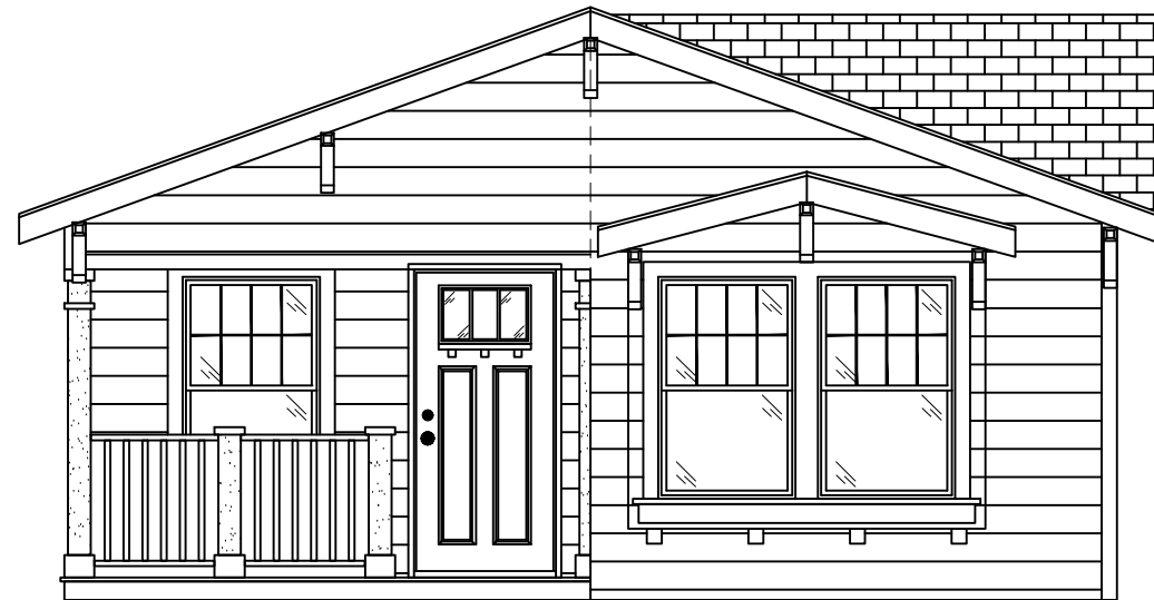
Front Elevation 4/12 Roof Pitch
