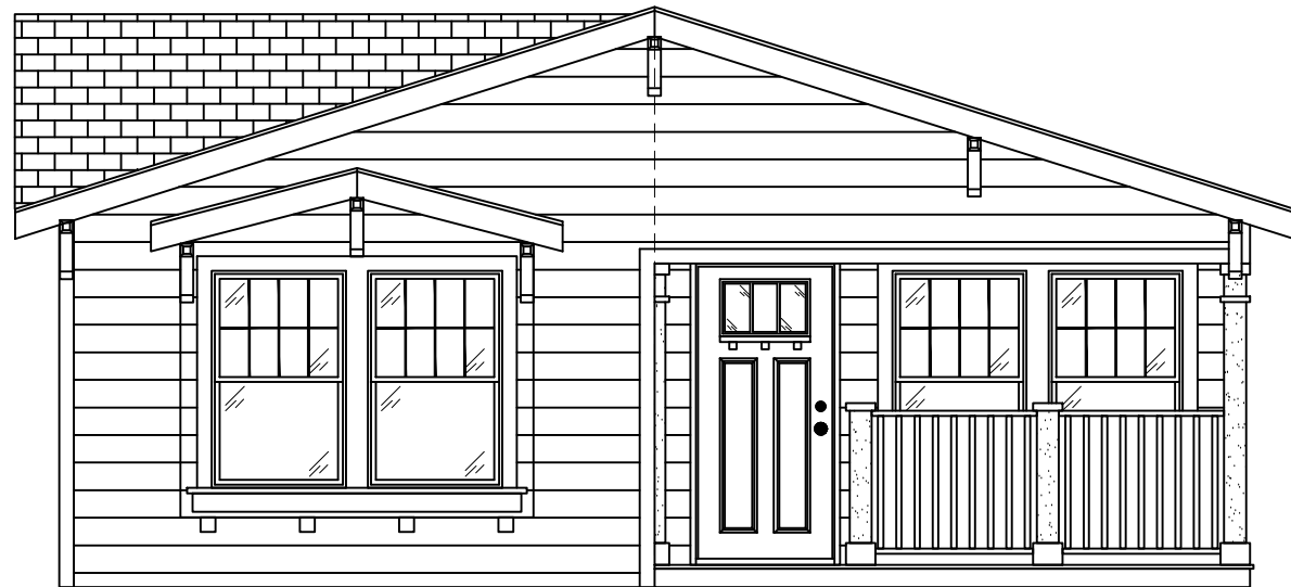
Front Elevation 4/12 Roof Pitch
