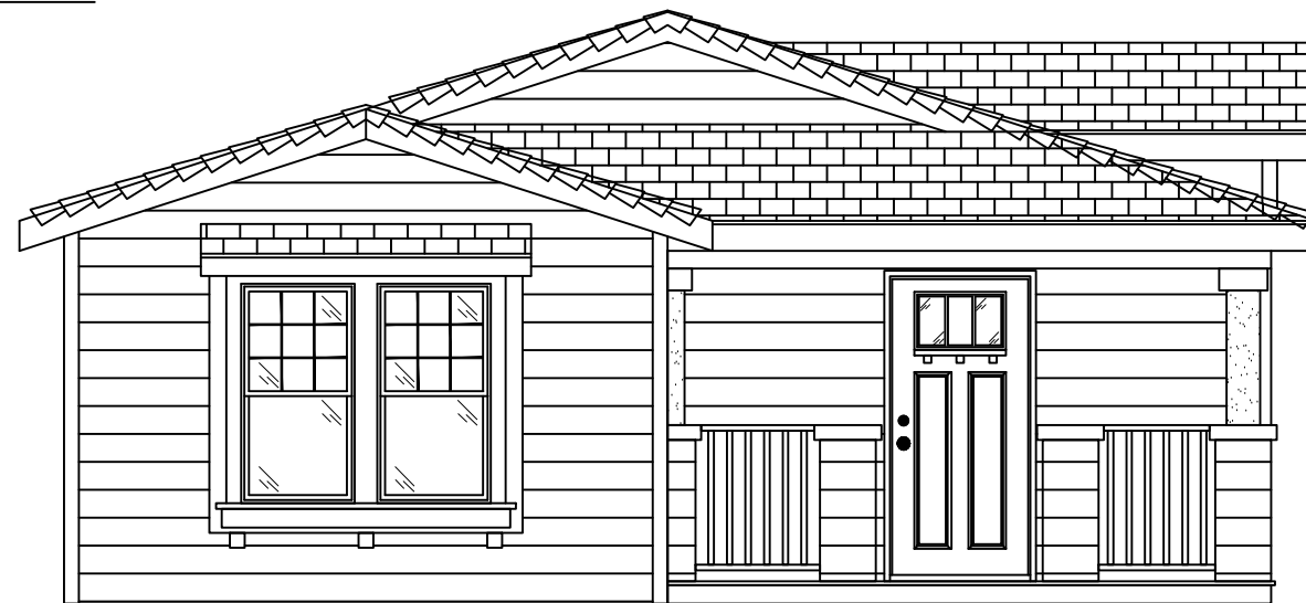
Front Elevation 4/12 Roof Pitch
