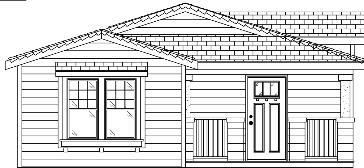
Front Elevation 4/12 Roof Pitch
