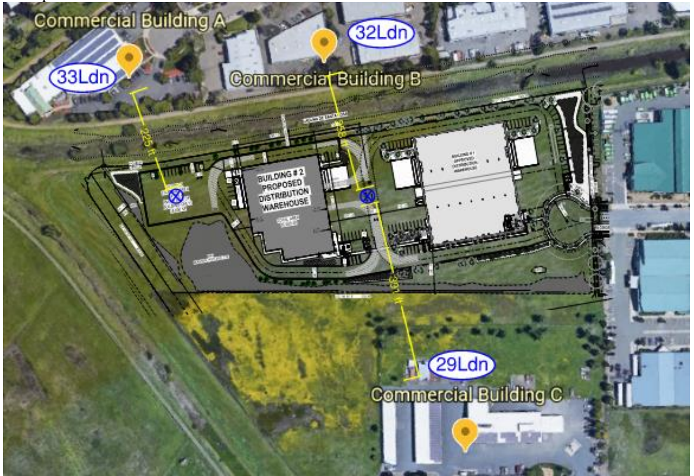
Figure 1: Approximate distances to nearest property lines from center of yards where most operations are expected to take place
